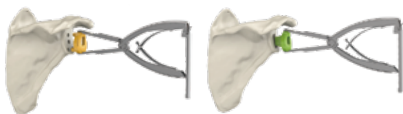
Grasp the Trial with the Glenoid Positioner and insert
